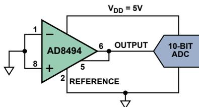
Figure 1. Simple thermometer.
