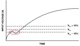
Figure 4. Nonmonotonic supply ramp.
