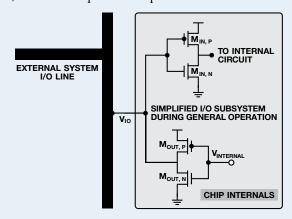
Figure 7. Simplified I/O circuit.
