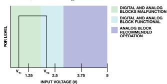
Figure 2. POR threshold voltages.
