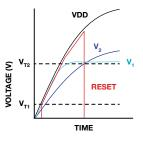
Figure 1. Simplified POR circuit.
