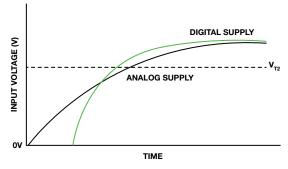
Figure 6. Recommended supply sequence.
