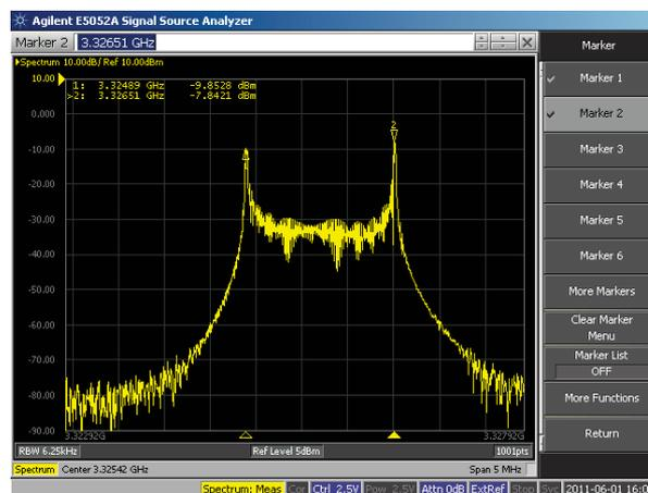
Figure 2. A spectrum-analyzer plot of ADF4350 VCO response to supply modulation by a 10-kHz, 0.6-V p-p square wave.
