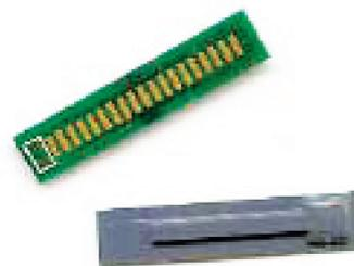
Figure 1. AT77C104B FingerChip IC.
