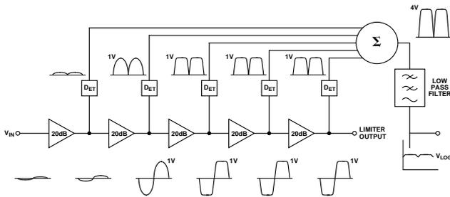
After the signal has gone into limiting in one of the stages (this happens at the output of the third stage in the figure), the limited signal continues down the signal chain, clipping at each stage and maintaining its 1 V peak amplitude as it goes.
