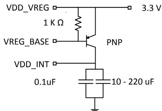
Figure 1. Voltage Regulator External Circuitry Design
